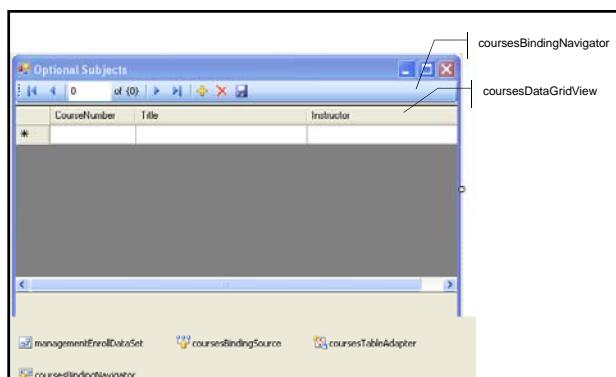
A **DataSet**, **BindingSource**, **TableAdapter**, **BindingNavigator** appear in the component tray. A **DataGridView** control and a tool strip for navigating records appear on the form.
