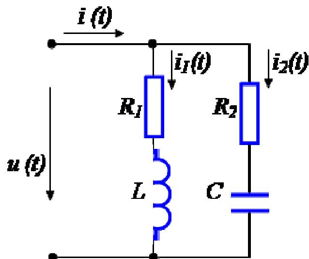
$$\omega_p = \frac{1}{\sqrt{LC}} \sqrt{\frac{{R_1}^2 - \frac{L}{C}}{(R_2^2 - \frac{L}{C})}}$$
