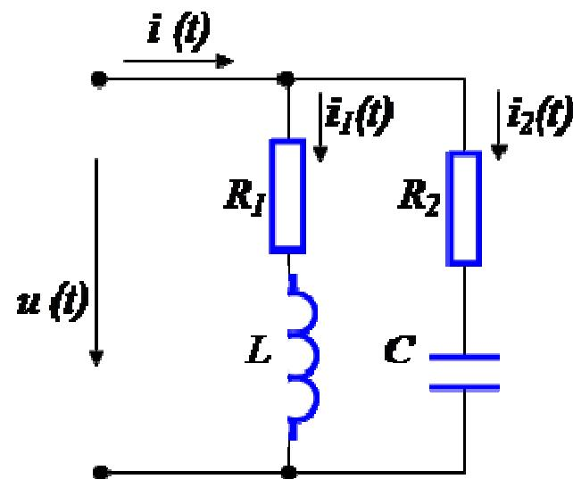
$$\frac{\omega L}{R_1^2 + \omega^2 L^2} = \frac{1 / \omega C}{R_2^2 + \frac{1}{\omega^2 C^2}} \quad (1)$$
