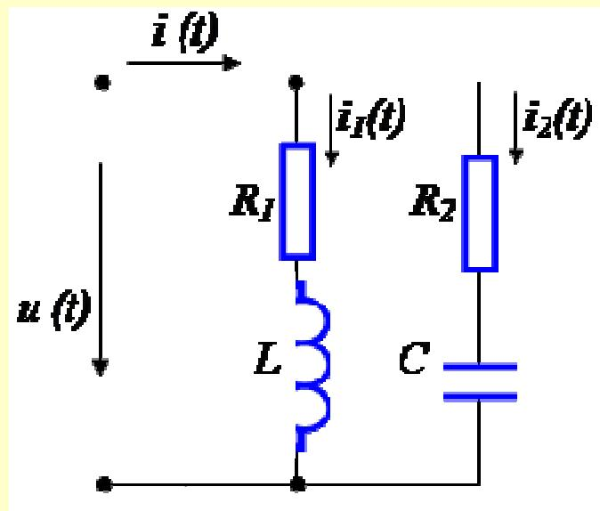
$$B_{екв} = \frac{\omega L}{R_1^2 + \omega^2 L^2} - \frac{1/\omega C}{R_2^2 + \frac{1}{\omega^2 C^2}} = 0$$
