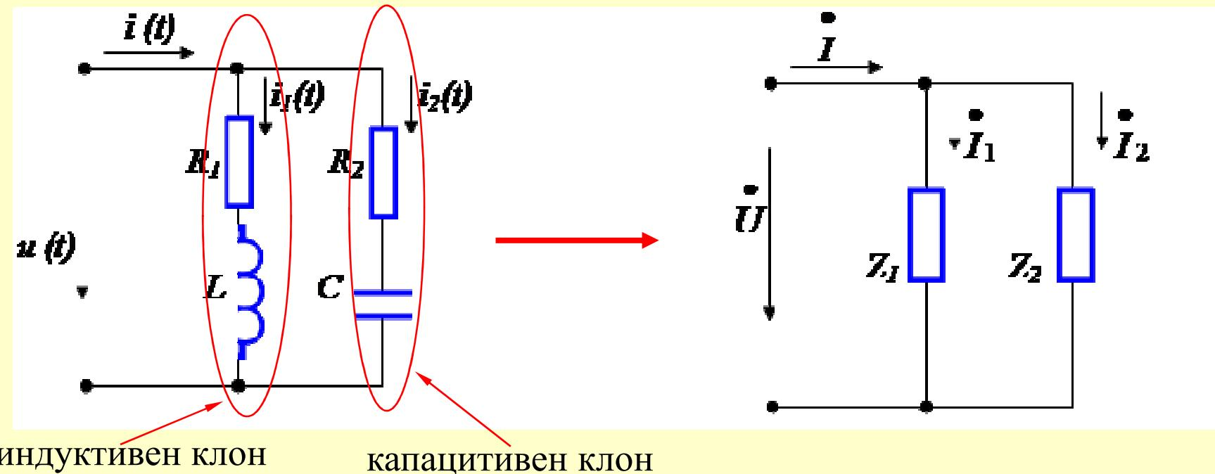
$$\overset{\bullet}{I} = \overset{\bullet}{I}_1 + \overset{\bullet}{I}_2 = \overset{\bullet}{U}(Y_1 + Y_1) = \overset{\bullet}{U} Y_{екв} = \overset{\bullet}{U}(G_{екв} - jB_{екв})$$
