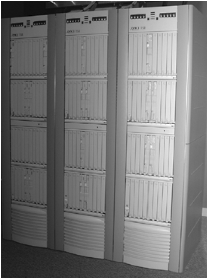
Figure 9.5 The Avici TSR is a scalable Internet router that uses a 3-D torus interconnection network as its switching fabric. Each cabinet holds 40 line cards, each of which provides up to 5 Gbits/s of interface capacity, arranged as a 2 \times 4 \times 5 sub-torus. Additional cabinets can be added to scale the machine to an 8 \times 8 \times 5 torus.
