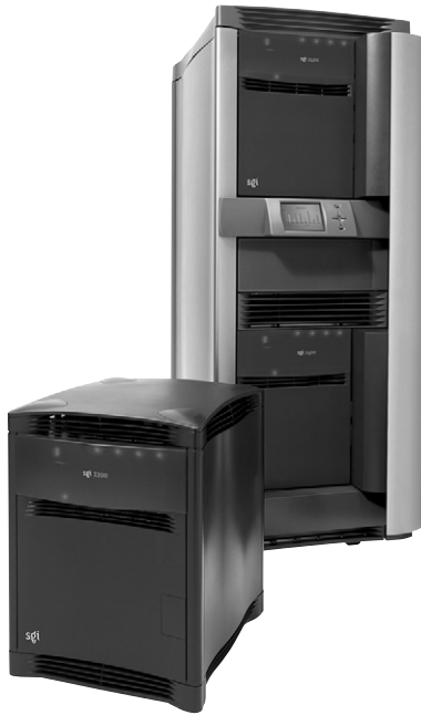
Figure 3.10 SGI Origin Servers. A single cabinet (16-processor) and a deskside (8-processor) configuration are shown.
