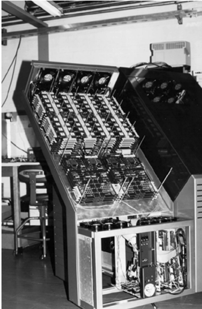
Figure 5.10 A pair of J-Machines. The near machine has its skins removed. The upper portion of the machine houses up to 1,024 processing nodes connected in an 8 \times 8 \times 16 mesh. This machine is half populated with eight 8 \times 8 64-processor boards. Below the processor array are I/O cards for graphics, disk control, and LAN interface. The bottom of the machine houses an 80-disk disk array.
