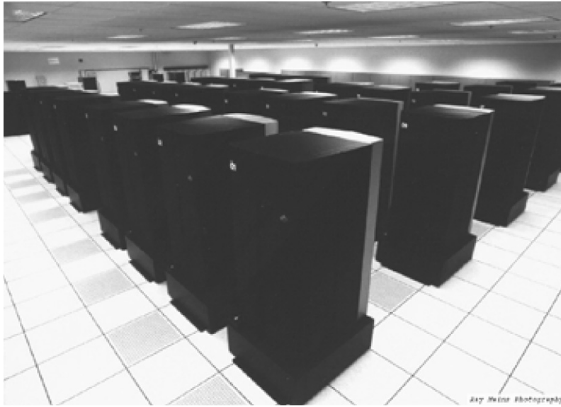
Figure 11.5 A 512-processor IBM SP2 system. Each cabinet, or frame, holds 16 RS6000 workstations and one 32-port switch board.
