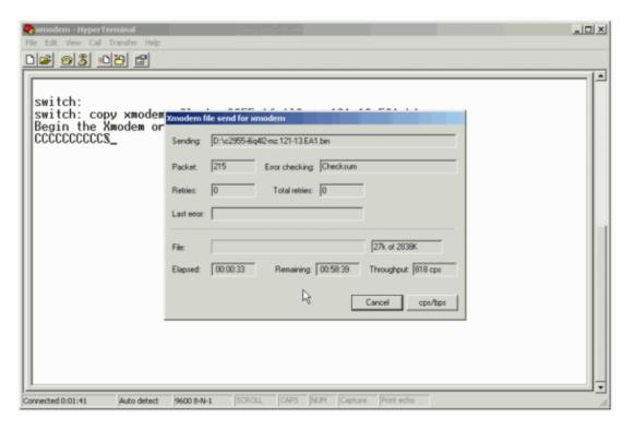
The Xmodem file transfer begins. This transfer can take up to 2 hours, which depends on the size of the image.
