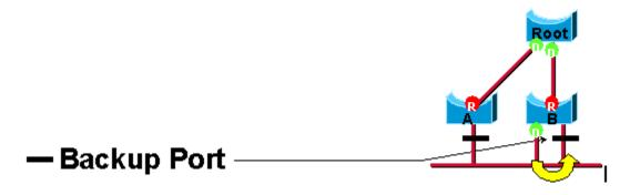
This distinction is already made internally within 802.1D. This is essentially how Cisco UplinkFast functions. The rationale is that an alternate port provides an alternate path to the root bridge and therefore can replace the root port if it fails. Of course, a backup port provides redundant connectivity to the same segment and cannot guarantee an alternate connectivity to the root bridge. Therefore, it is excluded from the uplink group.
