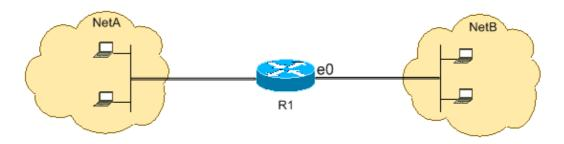
Telnet uses TCP, port 23. This configuration shows that all TCP traffic destined to NetA for port 23 is blocked, and all other IP traffic is permitted.
