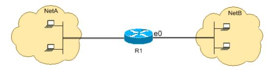
This configuration permits only echo–reply (ping response) packets to come in on interface Ethernet 0 from NetB towards NetA. However, the configuration blocks all echo–request ICMP packets when pings are sourced in NetB and destined to NetA. Therefore, hosts in NetA can ping hosts in NetB, but hosts in NetB cannot ping hosts in NetA.
