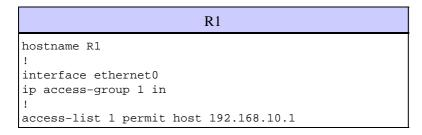
**Note:** The ACL filters IP packets from NetB to NetA, except packets sourced from NetB. Packets destined to Host B from NetA are still permitted.
