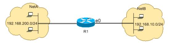
This configuration allows the IP packets with an IP header that has a source address in the network 192.168.10.0/24 and a destination address in the network 192.168.200.0/24 access to NetA. There is the implicit deny all clause at the end of the ACL which denies all other traffic passage through Ethernet 0 inbound on R1.
