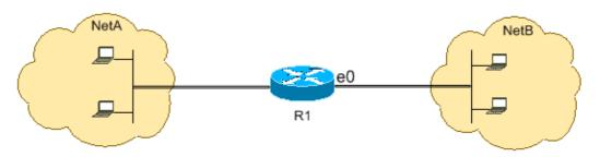
This configuration permits TCP traffic with destination port values that match WWW (port 80), Telnet (port 23), SMTP (port 25), POP3 (port 110), FTP (port 21), or FTP data (port 20). Notice an implicit deny all clause at the end of an ACL denies all other traffic, which does not match the permit clauses.
