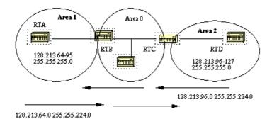
In the above diagram, RTB is summarizing the range of subnets from 128.213.64.0 to 128.213.95.0 into one range: 128.213.64.0 255.255.224.0. This is achieved by masking the first three left most bits of 64 using a mask of 255.255.224.0. In the same way, RTC is generating the summary address 128.213.96.0 255.255.224.0 into the backbone. Note that this summarization was successful because we have two distinct ranges of subnets, 64–95 and 96–127.
