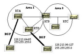
In the above diagram, RTA and RTD are injecting external routes into OSPF by redistribution. RTA is injecting subnets in the range 128.213.64–95 and RTD is injecting subnets in the range 128.213.96–127. In order to summarize the subnets into one range on each router we can do the following:
