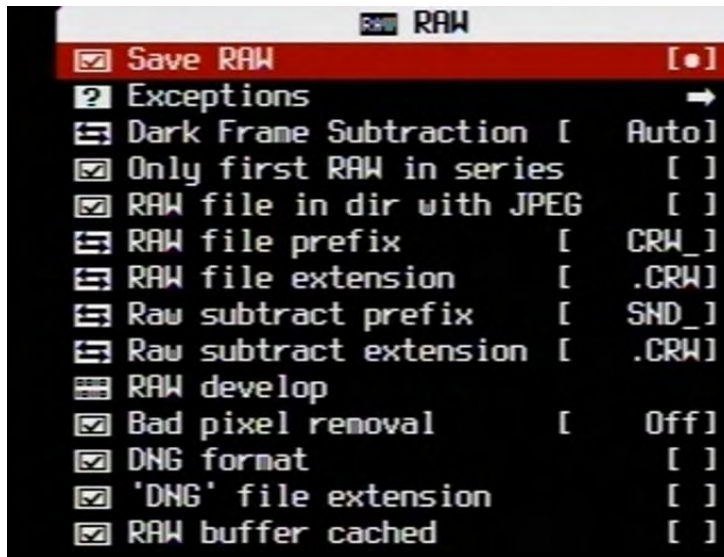
Figure 11-4. Enabling the Save RAW functionality in CHDK
