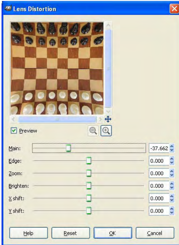
Figure 8-6. This image shows the results of applying too much pincushion distortion to correct a barrel distortion.
