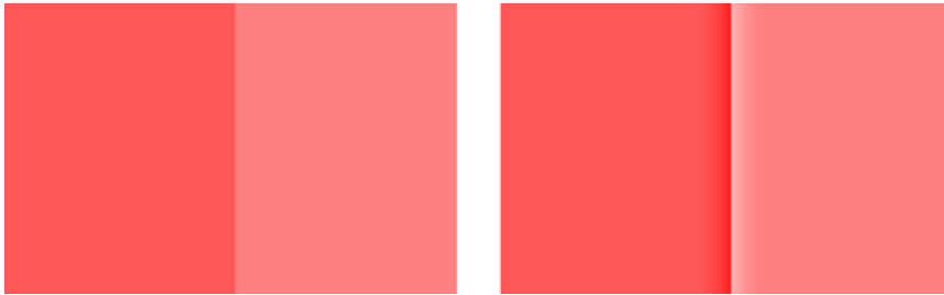
Figure 5-18. The right image shows the result of the Unsharp Mask over the left image. The contrast is enhanced in the edge, giving the illusion of a sharper image.
