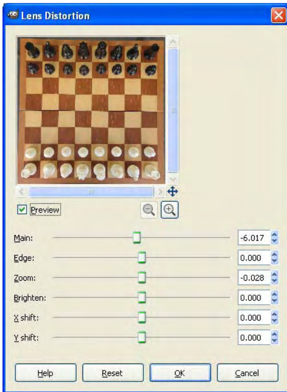
Figure 8-7. This image shows the settings used in the Lens Distortion dialog box in Gimp for correcting the barrel distortion.
