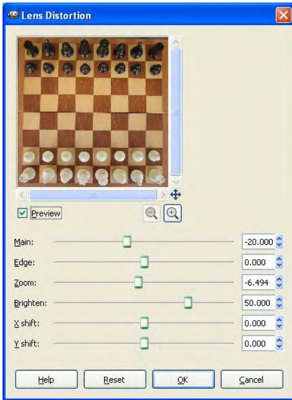
Figure 8-9. This image shows the parameters needed for reducing the effect of vignetting.
