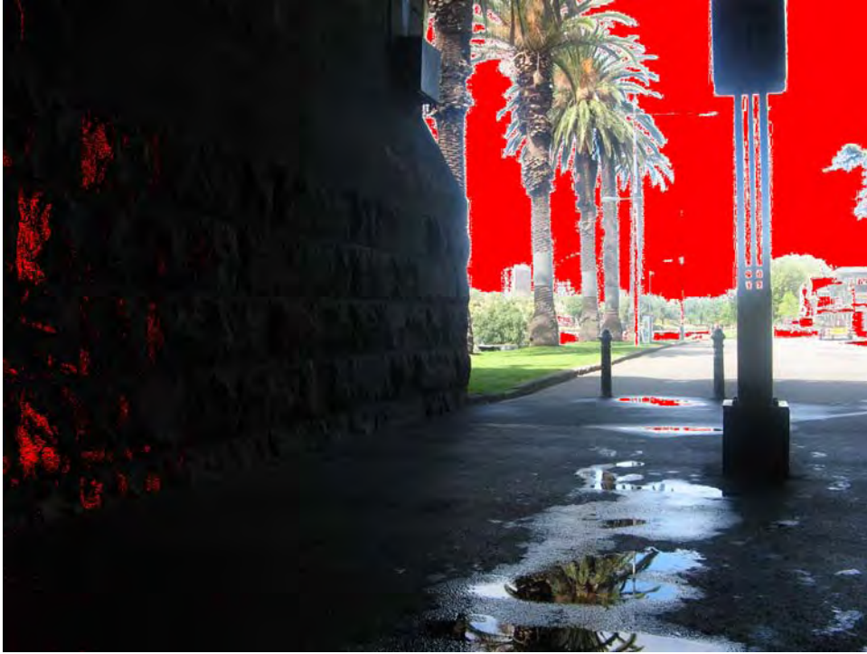
Figure 11-6. This image shows an example of the Zebra mode. This image seen in the LCD screen when the shutter button is half pressed shows a large overexposed portion due to the bright light marked in a solid color. Also, there is a small area underexposed on the left, also marked by the Zebra mode.
