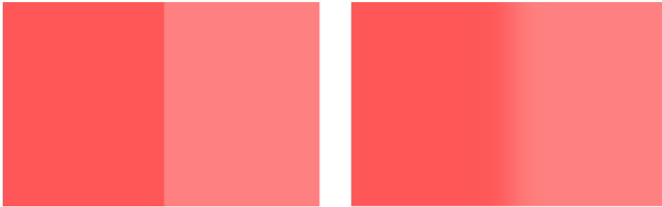
Figure 5-10. This image depicts a simple example of harsh borders. Note how visible the dividing line is in the left image. After applying a Gaussian blur, the dividing line is much less noticeable (right image).
