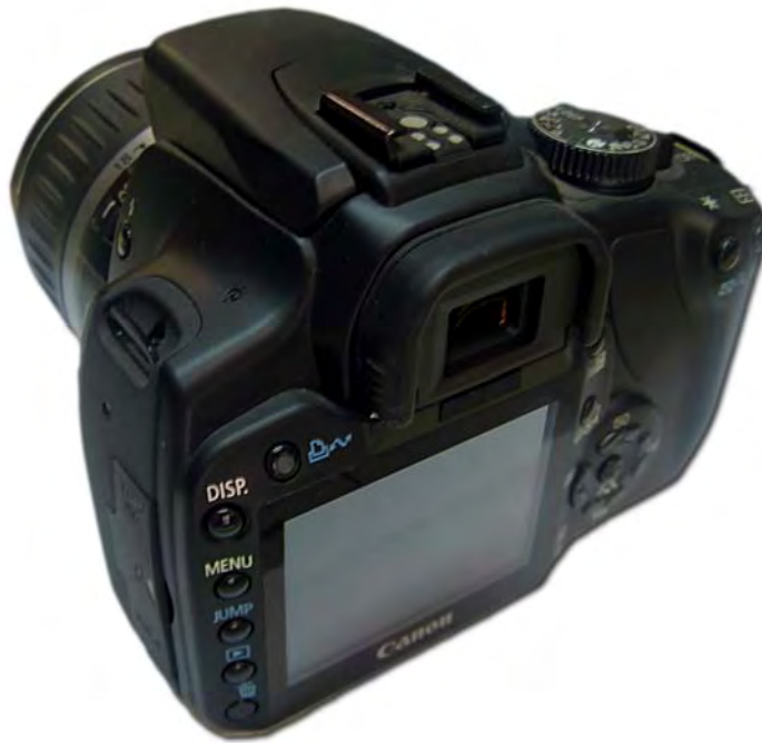
Figure 1-8. The back of a DSLR. You can see both the viewfinder (above) and the LCD screen (below) from this view.
