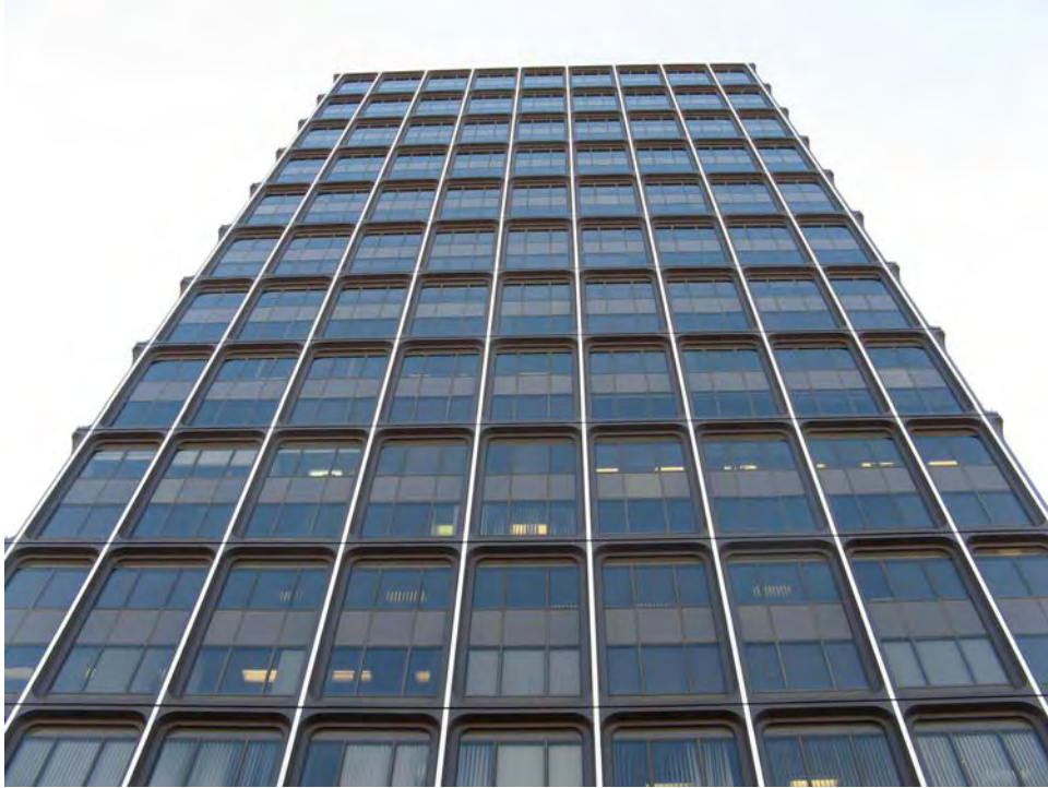
Figure 8-10. This image shows the original picture of a building. It clearly shows perspective distortion. Note how every floor appears as a different size in the image.
