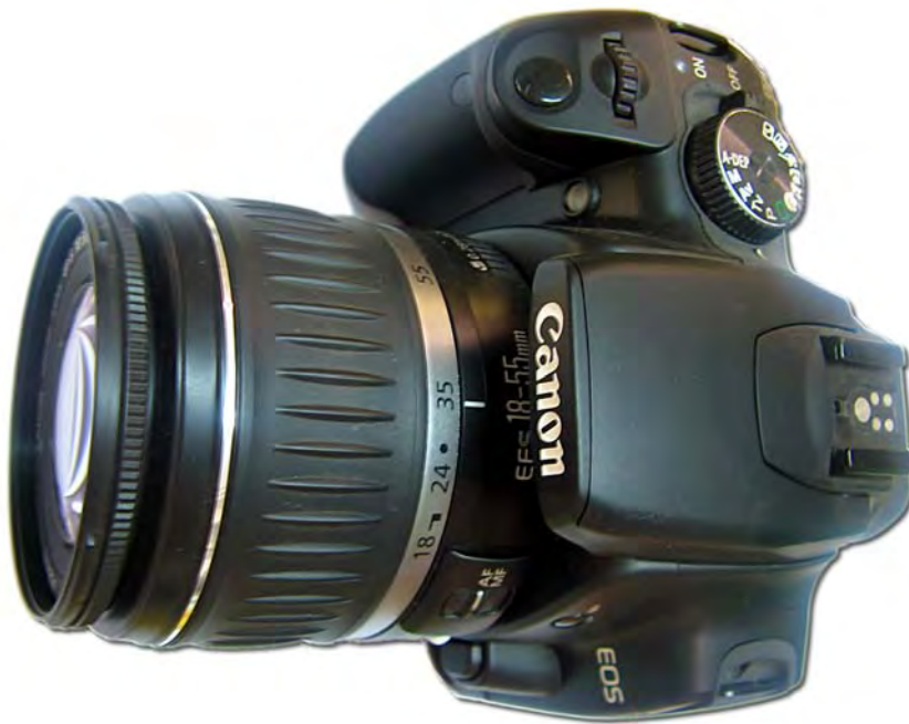
Figure 1-7. This image shows a digital single lens reflex camera with a lens mounted. This particular lens allows changing the focal length from 18 to 55 mm. The currently selected focal length is 35 mm.
