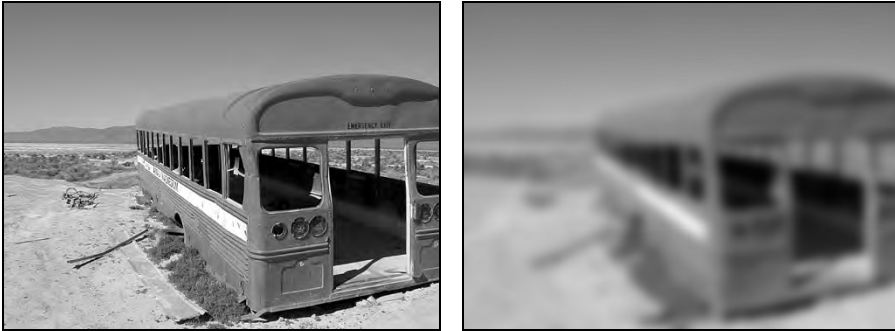
Figure 5.1 No point operation can blur or sharpen an image. This is an example of what filters can do. Like point operations, filters do not modify the geometry of an image.
