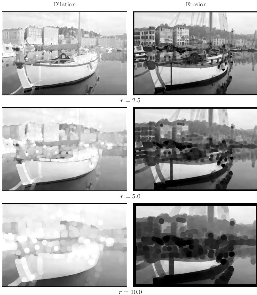
Figure 7.21 Grayscale dilation and erosion with disk-shaped structuring elements. The radius r of the structuring element is 2.5 (top), 5.0 (center), or 10.0 (bottom).
