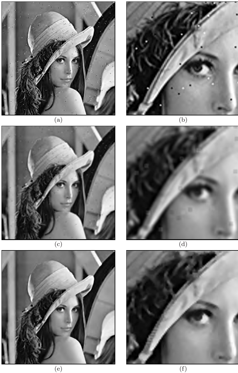
Figure 5.18 Linear smoothing filter vs. median filter. The original image is corrupted with “salt-and-pepper” noise (a, b). The linear 3 \times 3 pixel box filter (c, d) reduces the bright and dark peaks to some extent but is unable to remove them completely. In addition, the entire image is blurred. The median filter (e, f) effectively eliminates the noise dots and also keeps the remaining structures largely intact. However, it also creates small spots of flat intensity that noticeably affect the sharpness.
