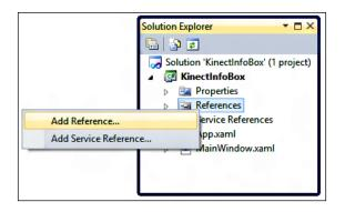
2. This will launch the Add Reference window. Then, search for the Microsoft. Kinect.dll file within the Kinect SDK folder. Select Microsoft.Kinect.dll and click on OK, as shown in the following screenshot:
