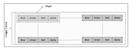
The previous diagram is the representation of each pixel within an image frame. The maximum value of each color is 255 and the minimum is 0. The following screenshot shows the color values for blue, green, and red along with the alpha values from an image frame:
