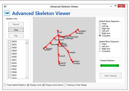
The sample project Hand Tracking with Joint Position Display is available for download in the book's resource location. This will work for both the seated and default modes and you see different bone sequences by selecting bone options. Record and playback is available for a fixed number of frames (limited to 1000 skeleton frames). Click on **Start Tracking** to start tracking the skeleton.
