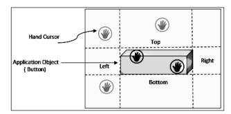
The preceding image illustrates how the hand cursor can identify the object. The complete backend logic is based on the coordinate system. The hand cursor will have a position that will keep changing with every skeleton frame. You will get the position of the hand cursor as CursorPoint by calling the GetCursorPoint() method of the HandCusror class.
