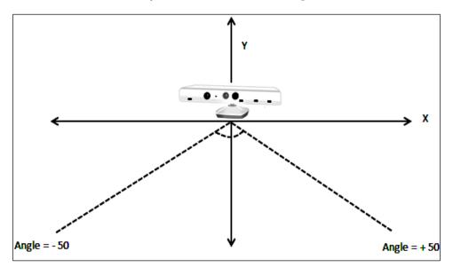
You can use the MaxSoundSourceAngle and MinSoundSourceAngle properties of the KinectAudioSource class to get the maximum and minimum values of the sound source angle.
