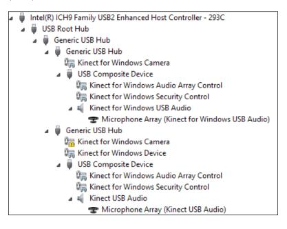
As the USB bandwidth is important, Kinect reserves the bandwidth for the camera for the first time when the drivers load. So, the first Kinect that is loaded will hold the bandwidth it needs. Then, any further connected Kinects will fail to load their camera drivers. Even if you aren't using the first loaded device, it will still hold the bandwidth for its own use. During unload, Kinect releases the bandwidth.
