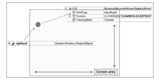
The overall representation of the skeleton data within global space is known as **skeleton space**. The origin of the skeleton space is the depth images that return the skeleton data with a set of joint positions. In the end, each joint position is represented with (x,y,z) coordinates. The ScalePosition() method, shown as follows, converts SkeletonPoint to DepthImagePoints, which is used as a mapping coordinate for the UI elements:
