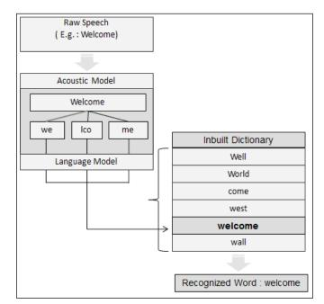
The following figure shows the basic speech recognition process using different modules of a speech recognizer:
