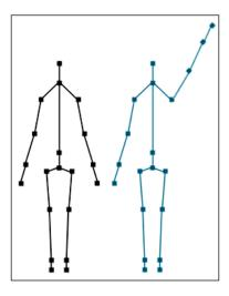
The Kinect for Windows SDK also supports tracking of a **seated skeleton**. You can change the tracking mode to detect a seated human body that returns up to 10 joint points, as shown in the following image:
