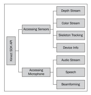
We can also define the SDK API as a **Natural User Interfaces** (**NUI**) API, which retrieves the data from the depth sensor and color camera and captures the audio data stream. There are several APIs that are written on top of the NUI APIs, such as those for retrieving sensor information just by reading sensor details and for tracking human skeletons based on the depth data stream returned from the sensor.
