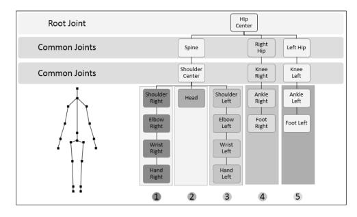
As shown in the previous diagram we can have a total five sequences of bones (1 to 5). We can move and orient the entire skeleton in the skeleton space by translating and rotating the root joint.
