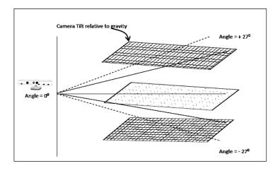
Do not physically force the device into a specific angle; allow the position to be set by your application automatically, as few times as possible.
