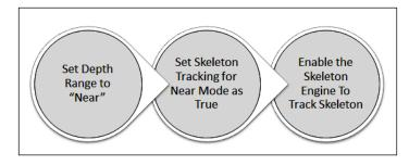
When we set the tracking range to Near, it is intended to track a player within a very close range. If you are building an application that tracks people very close to the Kinect, the best combination is seated-skeleton tracking with near mode tracking enabled.
