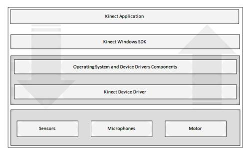
The installed drivers for the sensors sit with the components of system device drivers and can talk to each other. The drivers help to stream the video and audio data from the sensors and return it to the application. These drivers help to detect the Kinect microphone array as a default audio device and also help the array to interact with the Windows default speech recognition engine. Another part of the Kinect device driver controls the USB hubs on the connected sensor as well.
