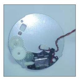
The motor can be tilted vertically up to 27 degrees, which means that the Kinect sensor's angles can be shifted upwards or downwards by 27 degrees. The following figure shows an illustration of the angle being changed when the motor is tilted:
