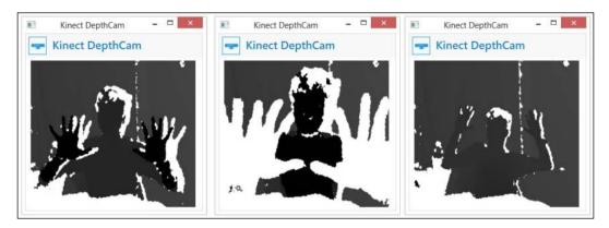
That was all about capturing the basic raw depth data from the Kinect sensor. So far you have enabled the depth stream and attached the event handler, which will invoke automatically whenever there is a depth frame. The frame will have the raw depth data that you need to handle within the depth frame ready event handler. So, let's have a look at the other properties and methods for the depth stream, which help to capture and process the data.
