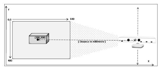
The viewable angle range will remain the same with the change of sensor elevation angle, as the change is considered as a change on the base of the Kinect sensor.
