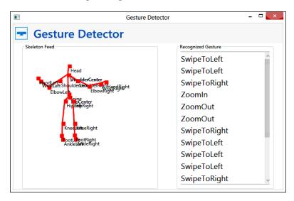
The working solution of the *gesture detector* is a sample project available in the GestureDetector folder of the resource location for this book. This application leverages the algorithmic gesture recognition engine we just built, and can detect four types of specified gestures. You will also be able to view the skeleton joints within this application.
