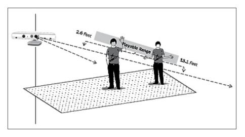
The Kinect depth sensor calculates distance based on the straight distance between the object and sensor. When there is a pixel in any of the diagonal views of the sensor, it internally draws a line that is perpendicular to the sensor and then calculates the distance directly from there, as shown in the following image:
