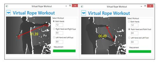
Calculating the distance between joints and performing the actions based on the value of the distance are examples of basic gestures to start with developing and understand how gestures work.
