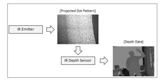
At this point, you might think, how does a single IR camera provide the depth information? How does the sensor get point information? There is an interesting concept behind this, which is known as stereo triangulation.
