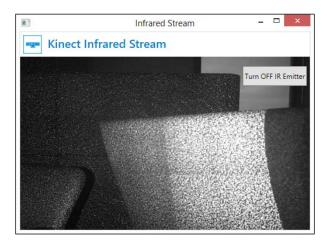
Apart from using the infrared stream to capture images in low light, you can use this to calibrate the cameras while you are using multiple Kinect sensors or using the Kinect camera with other camera devices.
