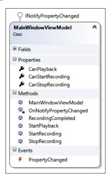
The MainWindowViewModel class also has a set of methods to enable and disable the UI buttons during start, stop, and playback of the recorded audio. For example, when we click on the **Start** button, it invokes the StartRecording() method, which sets the CanStartRecording and CanPlayback properties to false.
