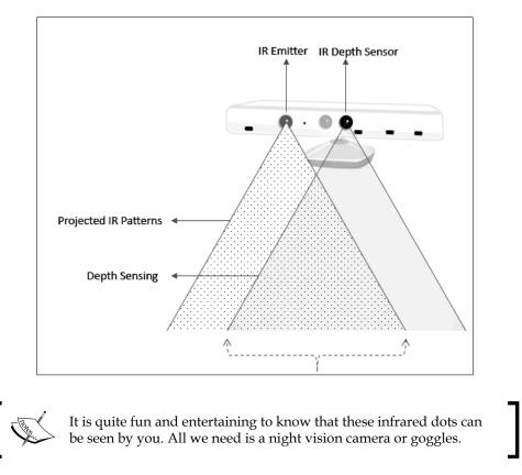
The depth data stream supports a resolution of 640 x 480 pixels, 320 x 240 pixels, and 80 x 60 pixels, and the sensor viewable range remains the same as the color camera.
