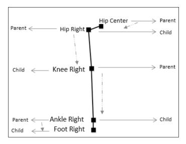
Parent joints drive the transformations of their respective child joints. Thus, when we translate or rotate a parent joint, we also need to translate or rotate all of its related child joints. For example, when one moves a knee joint, the child joint, that is, the knee also moves. However every joint has a degree of freedom, for example, a knee can only move in one direction, whereas a head can move in all directions.
