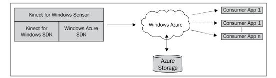
Now you can monitor location where you have placed the Kinect sensor and get the information you need from a URL. Your imagination is the only limit when developing applications based on this concept.
