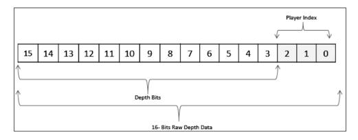
From the available 16-bit data, we need the upper 13 bits to get the distance. So, first of all we need to perform a **bitwise shift operation** (>>) to move the bits to their correct position.
