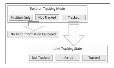
You can't add or remove any item from the joint collection. because JointsCollection in Skeleton does not implement an Add() or Remove() method. This is because it must always contain exactly 20 elements, corresponding to the 20 trackable body joints.
