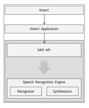
The **Speech Application Programming Interface** (**SAPI**) works as a middleware and provides an interface between the application and speech recognition engine.
