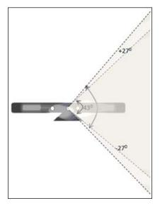
The default elevation angle is 0 degrees, which indicates that the sensor is pointing to a perpendicular gravity. So when the Kinect sensor is on the default angle, it considers a perpendicular gravity as the base. Changing the sensor angle involves just changing the base of the gravity with respect to the previous base, because the base depends on the gravity and not on the sensor base.
