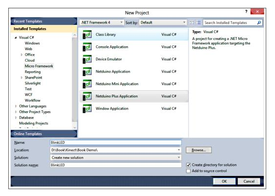
The default template for the Netduino Plus application contains all the assembly files required to start building an application. These references includes the required DLL files for the Microsoft .NET Micro Framework and the Netduino SDK. The following screenshot shows the added assembly (in Solution Explorer) and the used namespaces:
