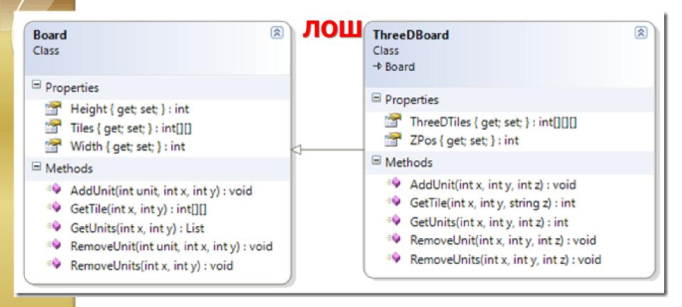
Instead of extending Board, ThreeDBoard should be composed of Board objects. One Board object per unit of the Z axis.
